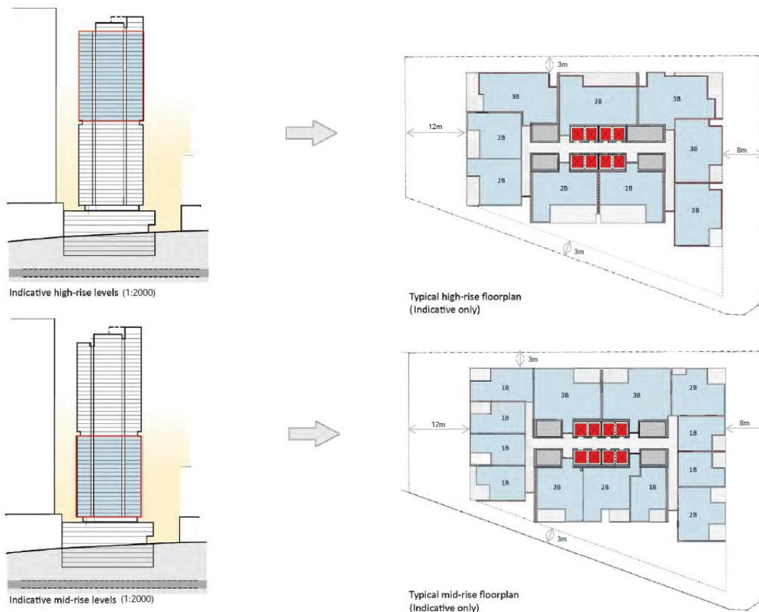
Figure 2: Typical tower floor plate (indicative only) source:
