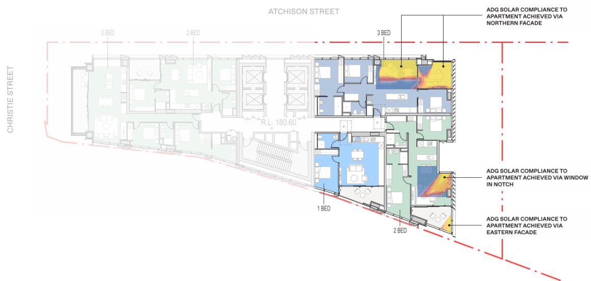
Figure 5: Solar Compliance – Eastern Units (Source: BVN Architects)
